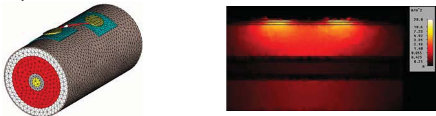
Figure 1: (left) Cylindrical multilayered model of the human upper limb, with tissue differentiation and excitation electrodes; (right) current density distribution across the structure at a given excitation instant (lateral view).
